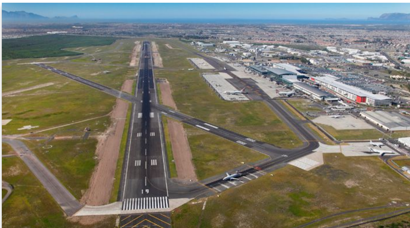
The approach onto Runway 19 will move 11.5 degrees counter clockwise to make way for the new R3.1bn runway 18/36. The old runway 19/01 is to become a parallel taxiway, the diagonal runway 16/34 is to be closed and disbanded
