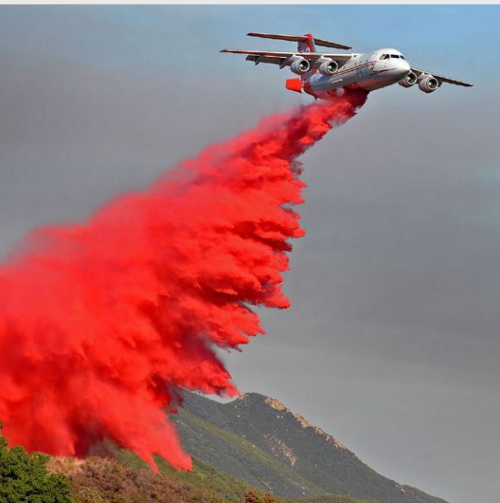
A 10 Tanker DC-10, '912' climbs away from the drop zone after dropping its 11,000 gallon load on a fire last September. The Albuquerque company used two Very Large Air Tanker (VLAT) DC-10s during the recent fires, but will soon have four available for 2018 fire-fighting season - 10 Tanker
